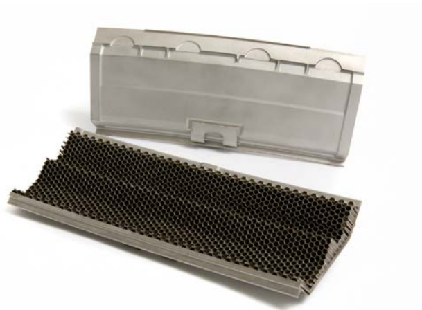
Low-pressure shrouds produced using space-saving, three-machine conventional EDM WorkMaster cells utilizing GF Machining Solutions' AgieCharmilles F0 350 and FORM 200 EDM machines
