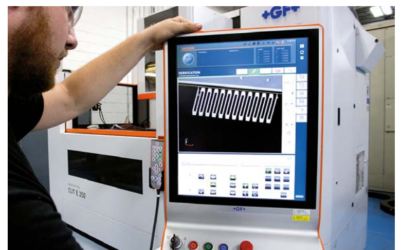
The AgieCharmilles CUT E 350's intelligent, intuitive AC CUT HMI puts fast, safe machining at EDM Supervisor Dave Coates' fingertips.
