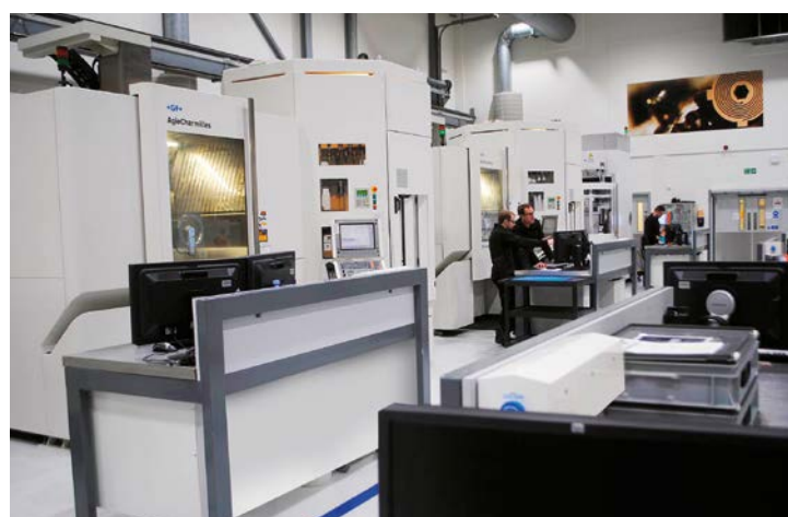
Much of the work to research, design, develop, manufacture and test the Mercedes AMG HPP hybrid PU is done by HPP's in-house Development Machine Shop, using technical partner GF Machining Solutions' high-performance Mikron Mill and AgieCharmilles wire-cutting EDM solutions.
