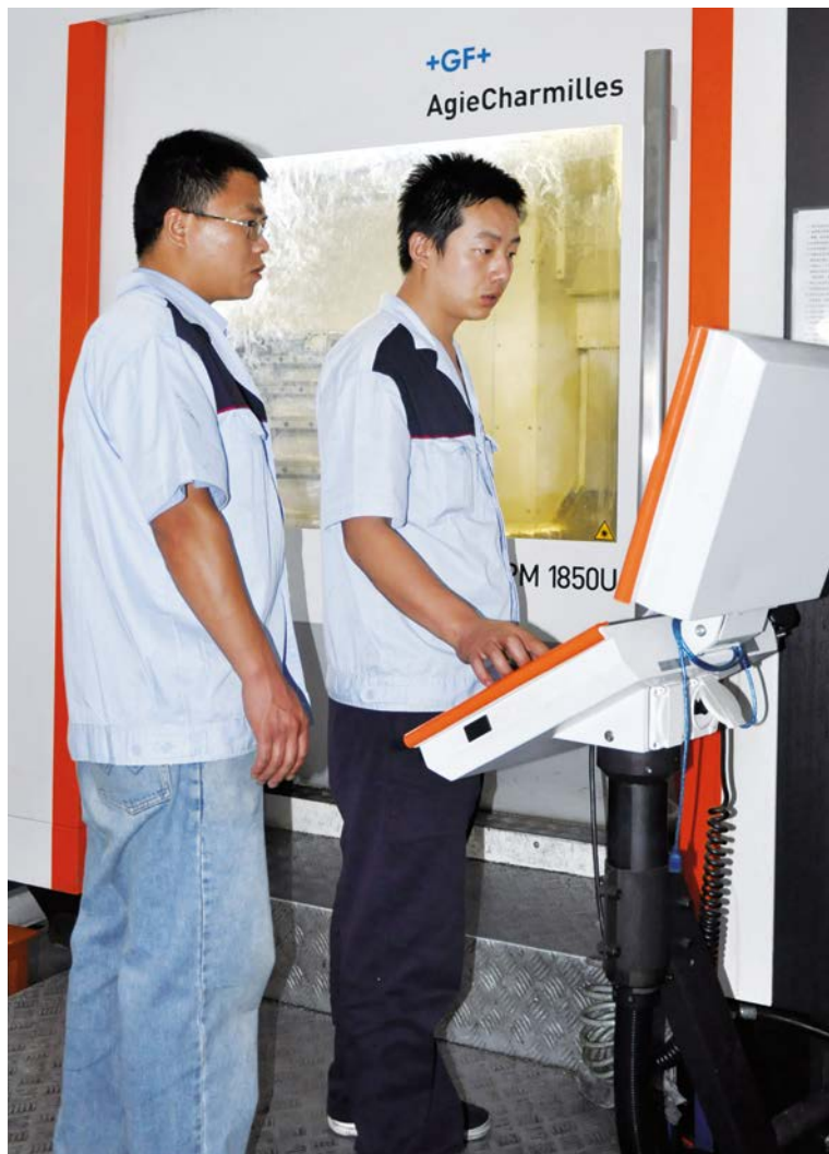
XTurbo machine operator Qipeng Ge (right) shows an apprentice how to use the Mikron HPM 1850U to machine large, difficult-to-cut aerospace parts.
